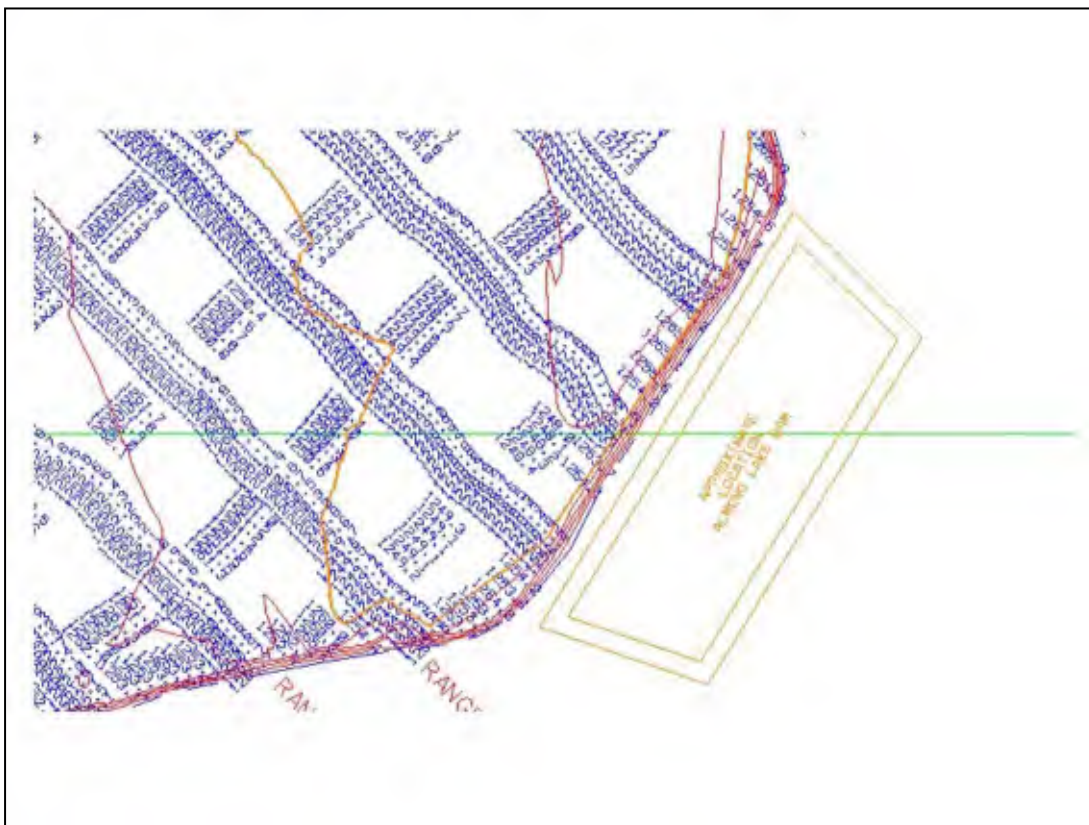
Figure L-4. Detail of survey vicinity Almond Lake Dam. 2-ft contours shown on drawings--1-ft contours used to compute storage capacities. (TVGA, Inc.)
